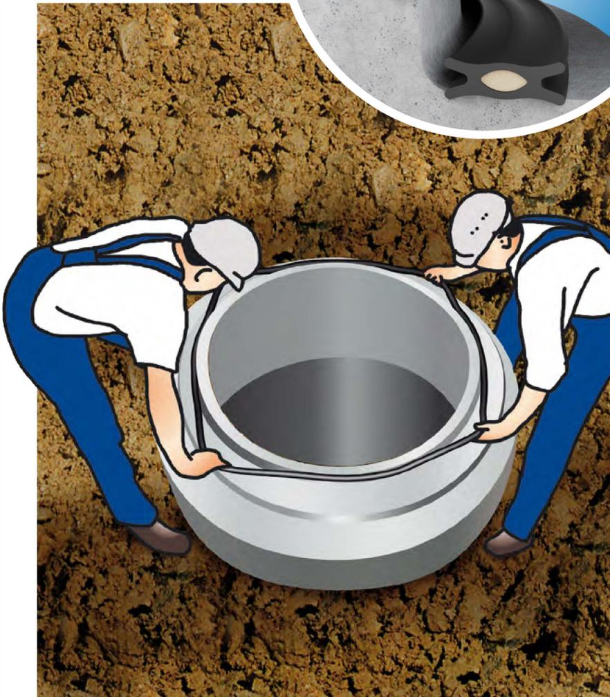
**1. Pull seal with mantle on top around on the cleaned spigot end, distribute tensioning evenly by repeated pulling at different spots.**
