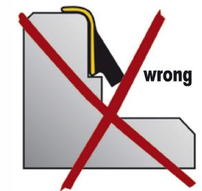
**2. Do not grease Belt or Seal, self-lubricating! Centre the manhole in the belt and hanging down straight and push manhole home. TOPSEAL Basic weight-balancing elements are a modern alternative for mortar**
